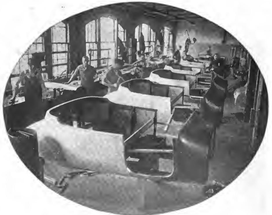
Where the metal-working is done. Bodies are of sheet aluminum
